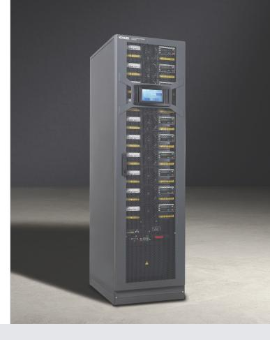
The KOHLER PW 8000DPA is a leading edge modular designed UPS using proven Decentralised Parallel Architecture (DPA) technology. The PW 8000DPA excels by offering broad load-range energy efficiency, "six nines" 99.999% availability and flexible scalability in either a tower or rack-mountable solution. The system offers high efficiency, low cost of ownership and a compact footprint that is proven in a wide range of critical applications.
