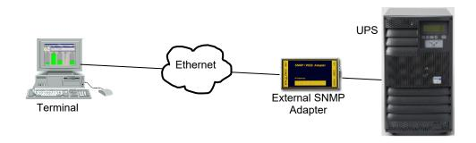
The external SNMP adapter is enclosed in a small box which must be powered from a backed-up supply supported by the UPS output so that its power is maintained in the event of a mains failure. A suitable plug-top power supply is included with the option kit.
