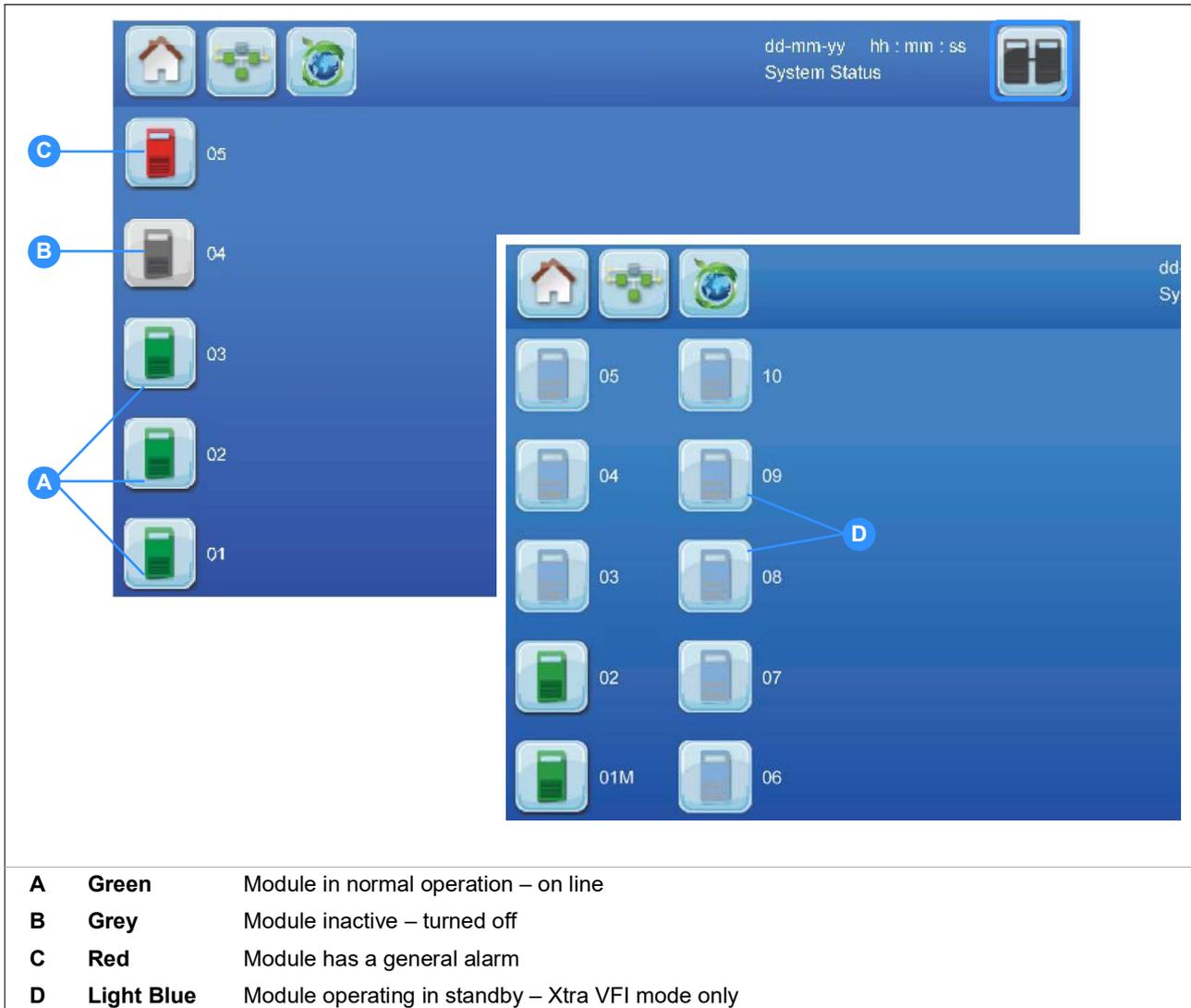
**Figure 3.19 Module selection display screen**
