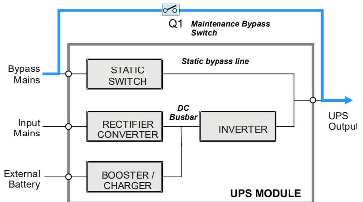
**Figure 2.8 Module OFF (Load on maintenance bypass)**
