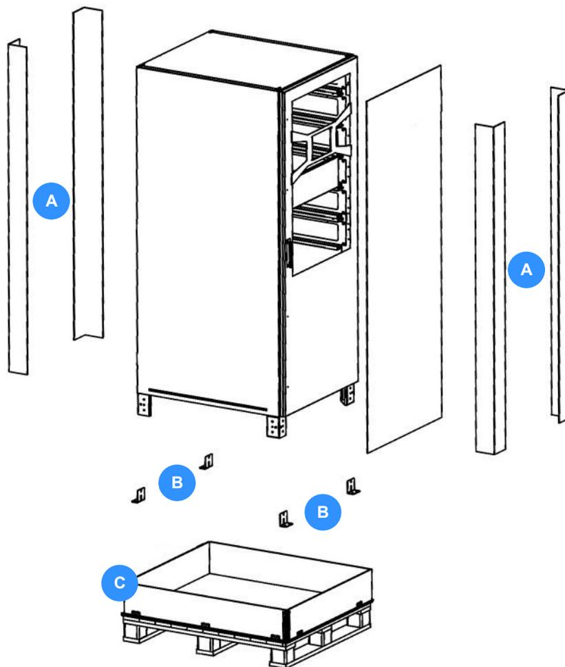
Figure 5.2 Unpacking the UPS cabinet (standard packaging)
