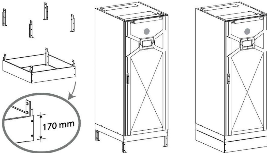
Figure 9.9 Elevation kit
