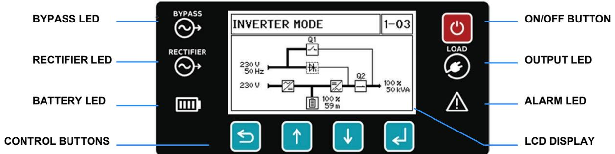
Figure 2.12 Module Control Panel
