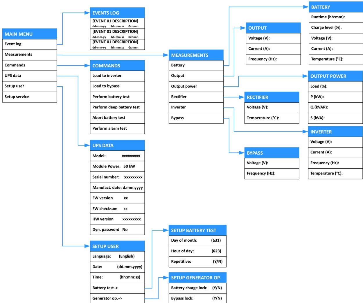
Figure 2.15 Module control panel menus
