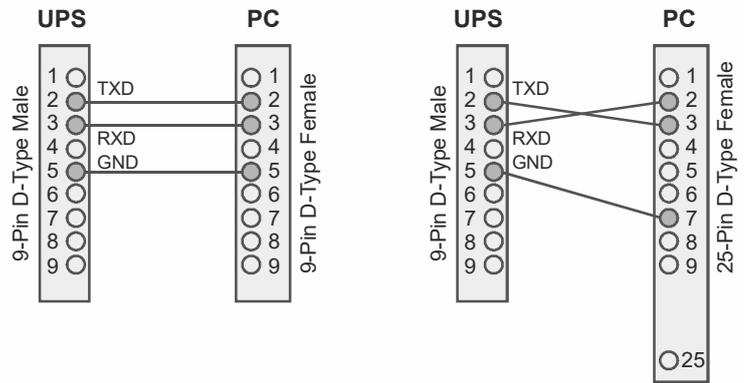
**Figure 9.8 Connector Cable - PC Serial Port**
