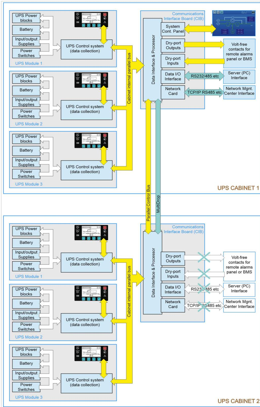
Figure 9.2 Inter-cabinet parallel connections
