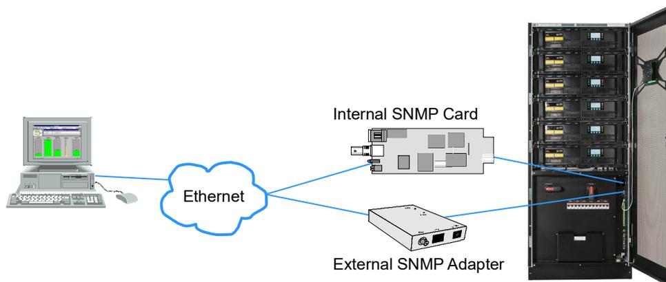
**Figure 1 SNMP Connection**
