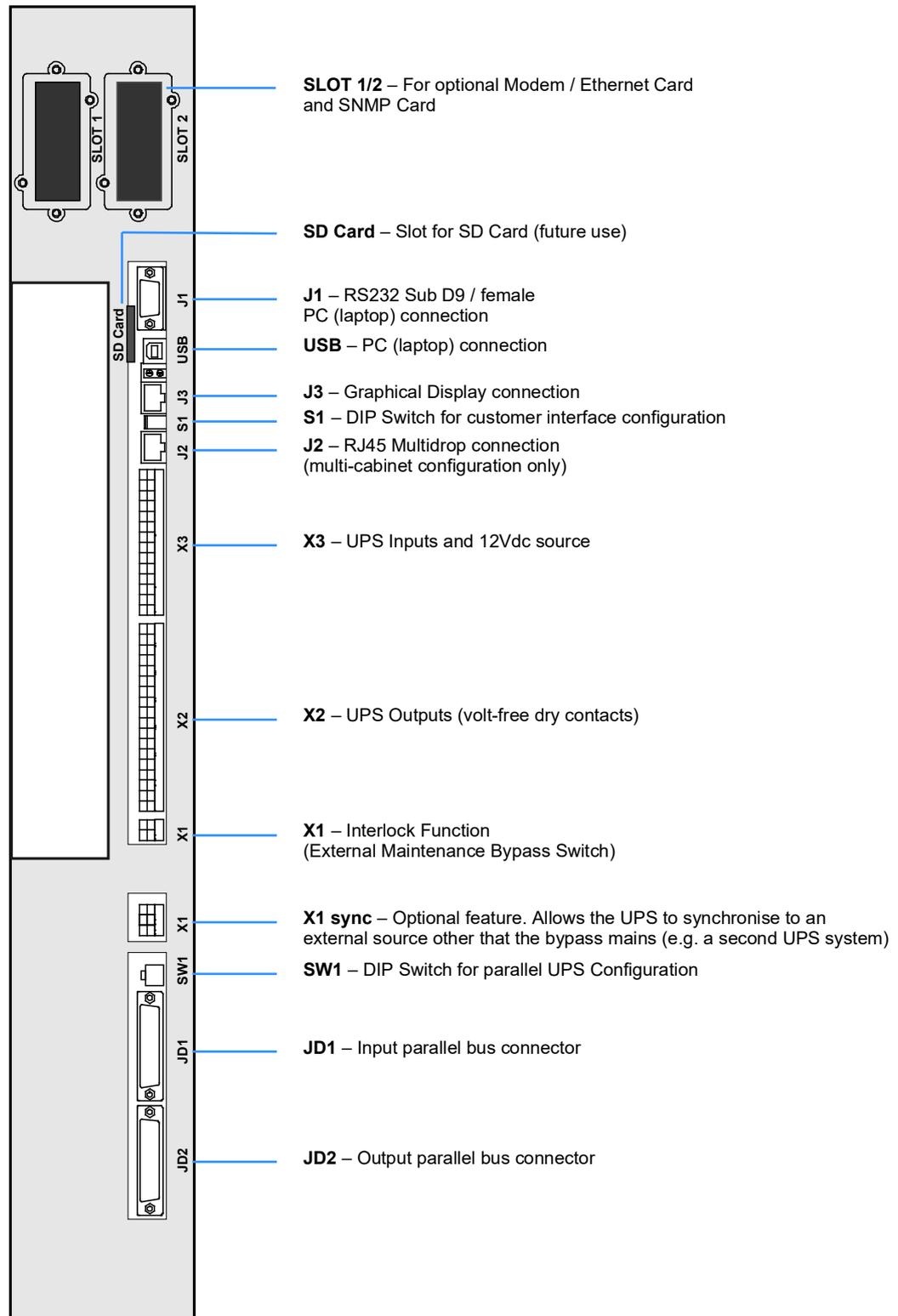
Figure 2.16 Customer interface board
