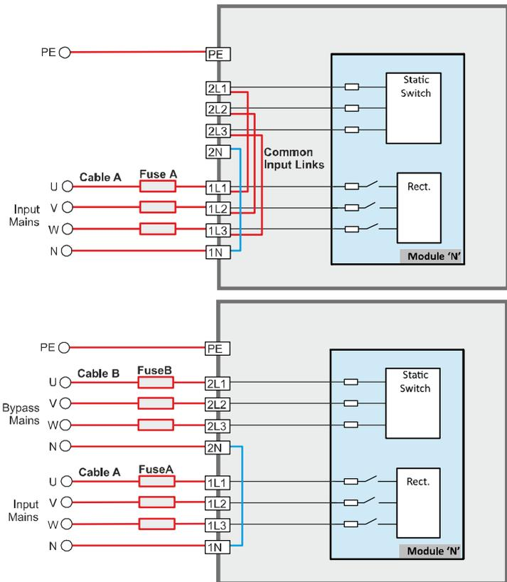
**Figure 4.4** Single and dual feed input configuration
