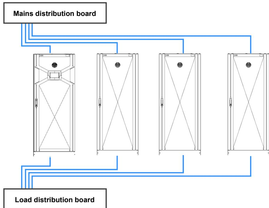
Figure 4.6 Cable lengths for multi cabinet configuration
