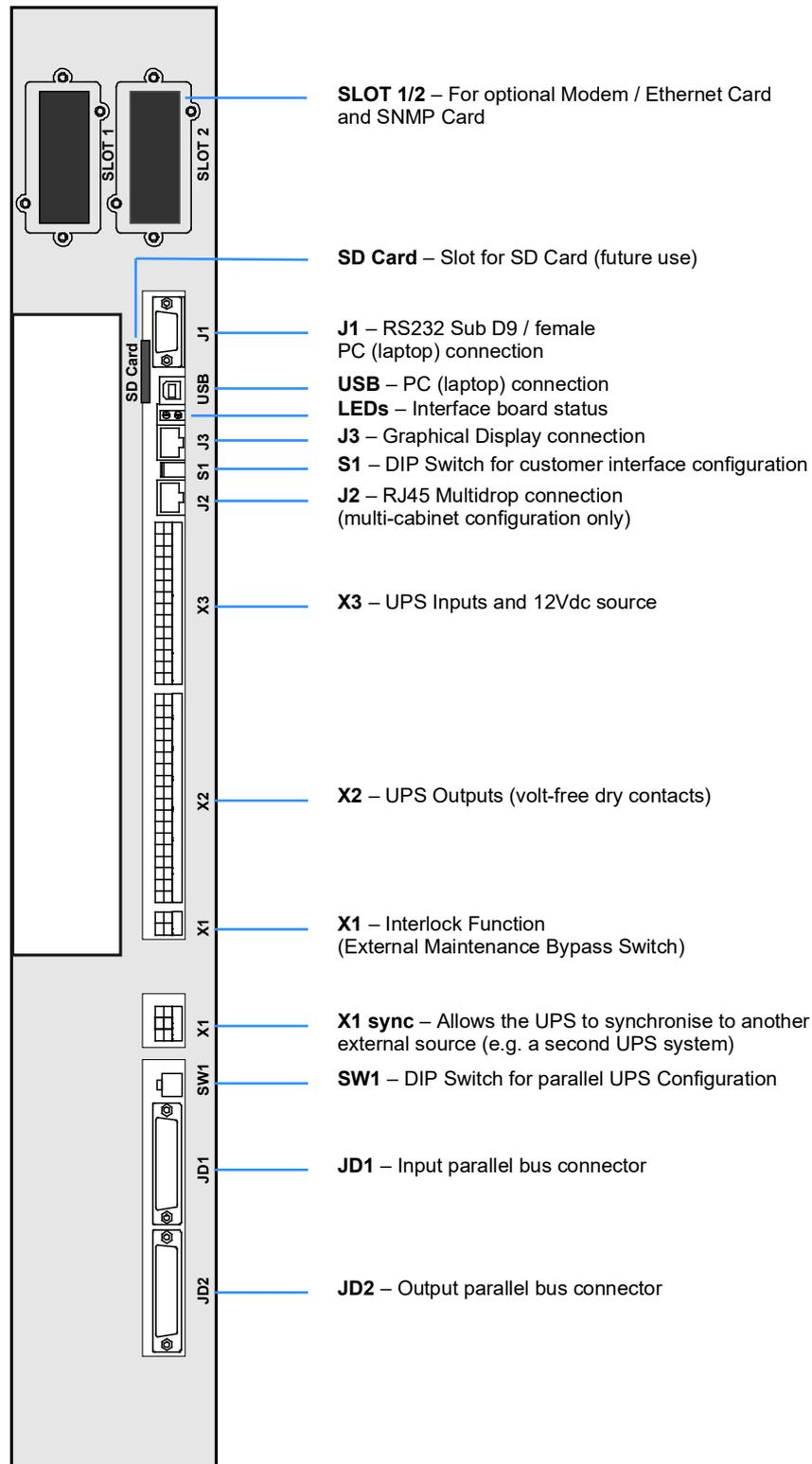
Figure 9.1 communications interface board
