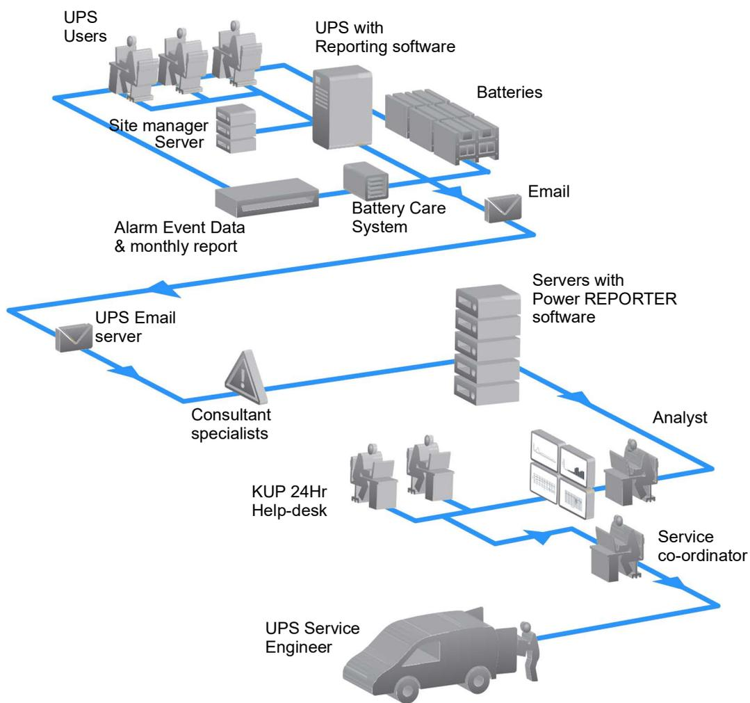
**Figure 2 Remote monitoring communications chain**
