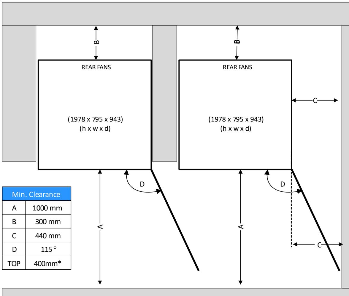
**Figure 4.1 Clearances for a Kohler PW 9250DPA (50-300 kW) stand-alone cabinet**
