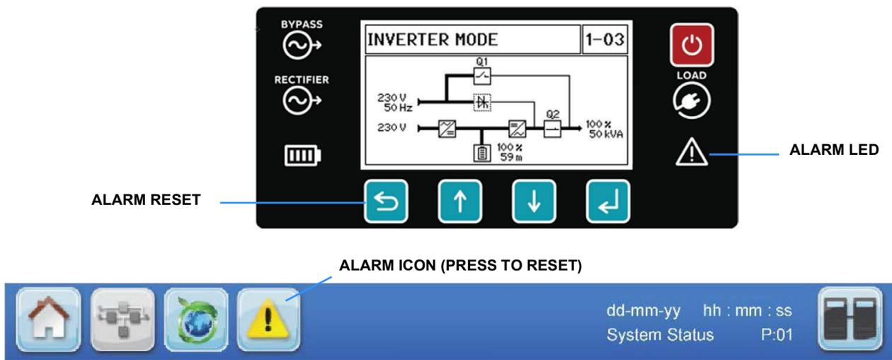
Figure 8.1 Control panel alarms
