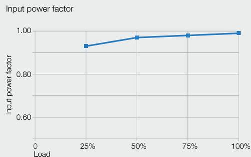
Near unity input power factor, at partial and full load, reduces the required size of the input cable and fuses, thereby reducing the materials (and costs) associated with the system's electrical installation.
