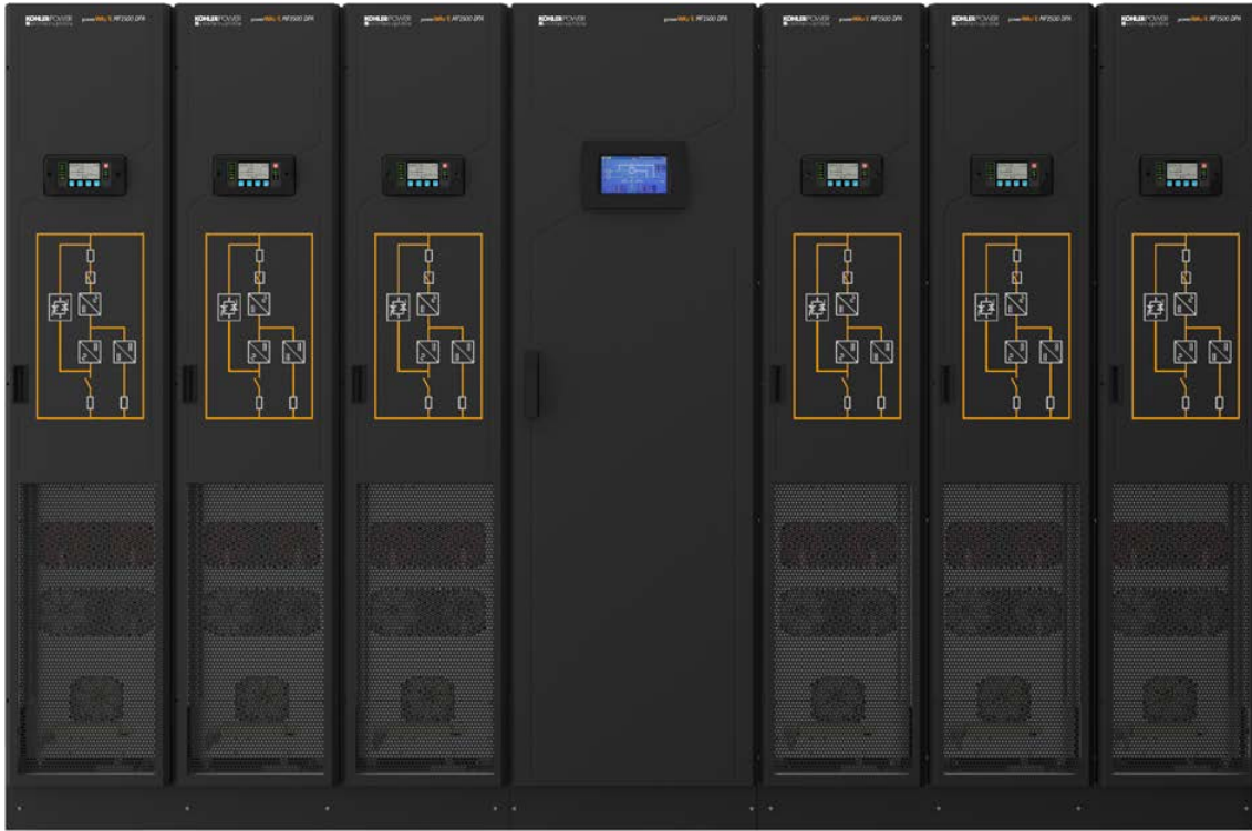
A 1.5MW MF1500 DPA with a central connections cabinet flanked by six 250kW modules, each containing all elements of a UPS.
