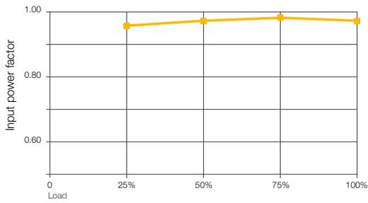
Near unity input power factor, at partial and full load, reduces the required size of the input cable and fuses, thereby reducing the materials (and costs) associated with the system's electrical installation.
