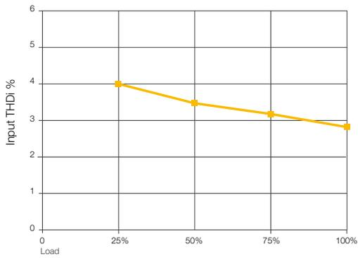
Input current total harmonic distortion (THDi) of <3% virtually eliminates harmonic distortion of the mains supply.
