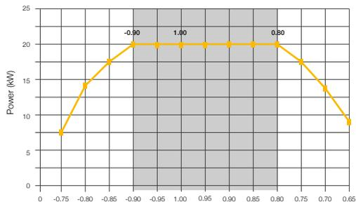
Fully rated output power in the range of 0.9 leading and 0.8 lagging
