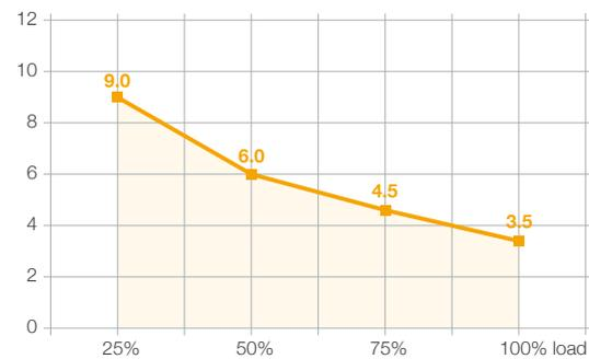
The PowerWAVE 6000 actively manages the input current total harmonic distortion (THDi) at a low level (3.5% at 100% load). PowerWAVE's unique technology neutralises the emission of harmonics at the input of the UPS system, providing greater reliability of operations for circuit breakers and extending the overall service life of the equipment.
