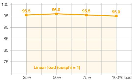
With a transformerless design and Energy Saving Inverter Switching (ESIS) technology, the PowerWAVE 6000 delivers high efficiency at partial and full load (up to 96.0% in double conversion online mode). This level of efficiency dramatically reduces the total cost of ownership of the UPS system during its life cycle.
