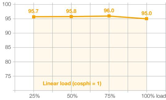
Top-of-market 96.0% efficiency in double conversion mode reduces running costs without compromising reliability. This UPS has a very flat efficiency curve so high efficiency is reached at low load levels.
