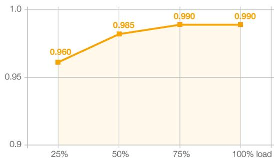
Thanks to the near-to-unity input power factor of 0.99, the PowerWAVE 6000 reduces the input installation costs by enabling the use of smaller cables. Furthermore, it avoids the unnecessary use of additional phase compensating devices, which consequently keeps the overall UPS efficiency high.
