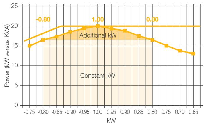
Designed to power all types of electrical loads including blade servers, the PowerWAVE 8000DPA can provide fully rated output power from 0.9 leading to 0.8 lagging.
