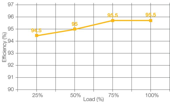
The PowerWAVE 8000DPA's 95.5% true online efficiency significantly reduces system running costs and site air-conditioning costs. This helps reduce the organisation's carbon footprint.
