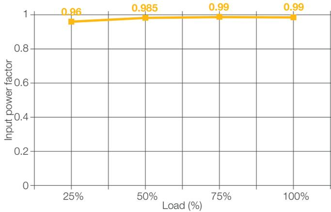
PowerWAVE 8000DPA has a near unity input power factor at full load (and even partial loads) reducing the size of the input cable and fuses, thereby saving on materials and costs.
