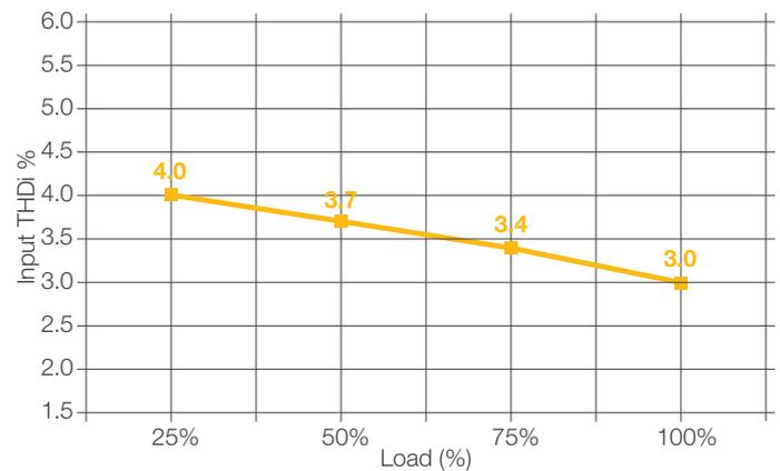
Input current total harmonic distortion (THDi) of <3% virtually eliminates harmonic pollution of the mains supply.
